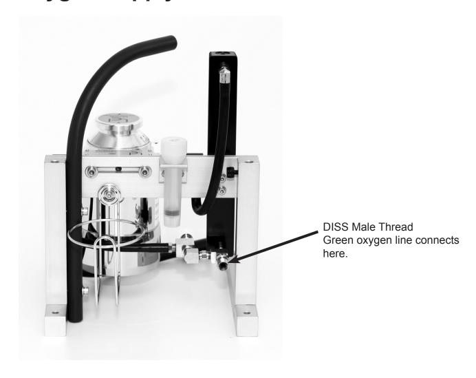
Attach the green oxygen hose to the DISS male thread.
